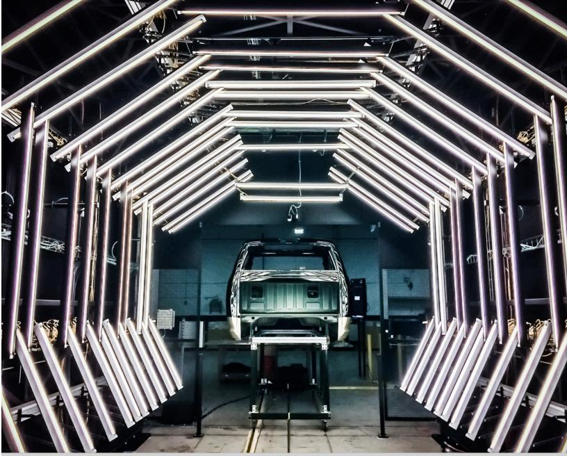
**Automotive Paint Defect Detection System**
